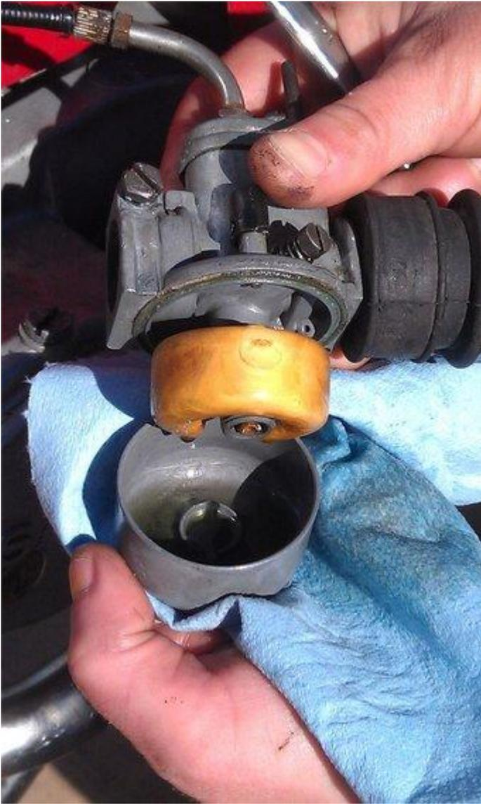
If you have a 14mm wrench, use that to loosen the float bowl. An adjustable wrench will also work. Once it's loose, you should be able to unscrew and remove it by hand. It might be full of gas, so hold the carburetor as straight as possible and have your rag handy.
