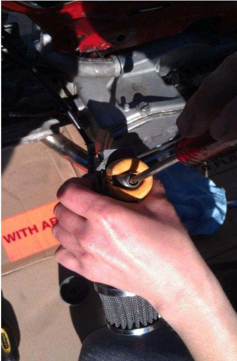
In the center of the carburetor is the jet. It's made of brass and is kinda delicate. Use a **SMALL FLAT SCREWDRIVER** to remove it. Be sure the screwdriver fits properly, or you'll mess up the jet. Seriously. **NOTE**, there is a chance that the jet will come out attached to a tube. No worries. Once it's out, use pliers or something to hold the tube, then remove the jet.
